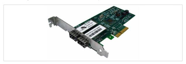
Apply two Gigabit Fiber SFP ports server connections in a single PCI Express \* slot.
